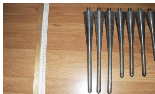
Figure 3. Models of semi-conical piles for tests with a head diameter d = 30 \text{ mm}
