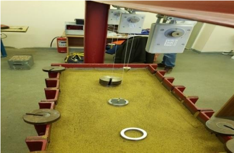
Figure 5. Fragment of tests of models of foundations of a round shape with through holes
