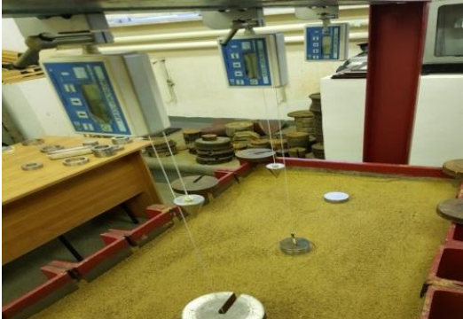
Figure 2 – A fragment of tests of models of foundations of a round shape
