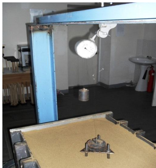
Figure 5. Test of the 3-pile cluster model
