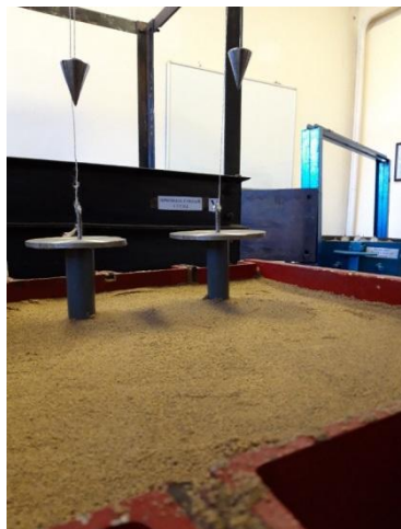
Figure 6. Beginning of step loading of the pile
