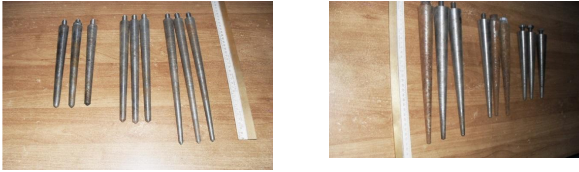
Figure 4. Models of conical piles for tests with a head diameter d = 20 mm
