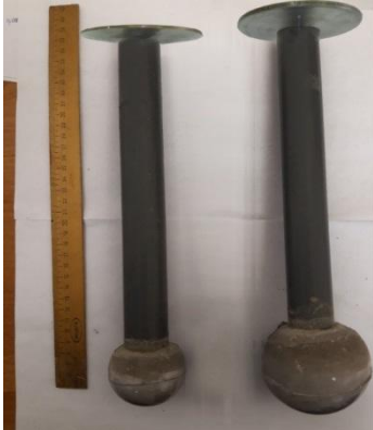
Figure 3. Models of bored pile with expanded base used in laboratory research, before testing
