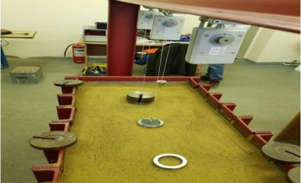
Figure 3 – Fragment of tests of models of foundations of a round shape with through holes
