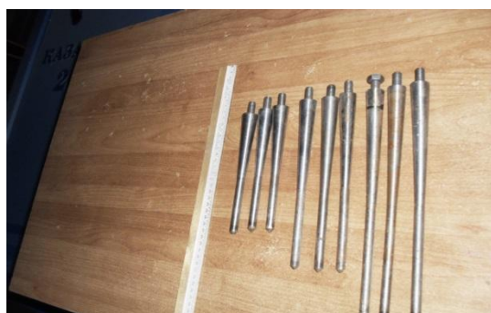
Figure 2. Models of semi-conical piles for tests with a head diameter d = 20 \text{ mm}
