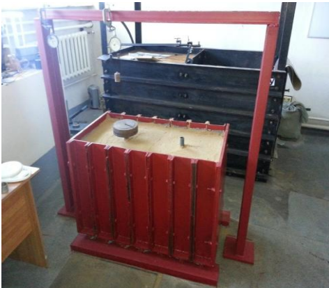
Figure 1. Volumetric stand in the laboratory «Geotechnics»
