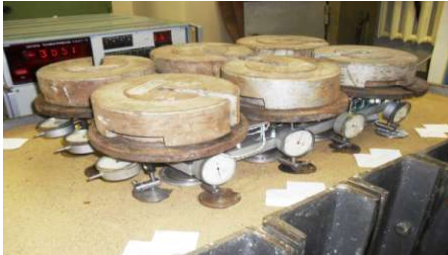
Picture 1. Tensometric system for the construction of conical foundations with a truncated base before testing.
