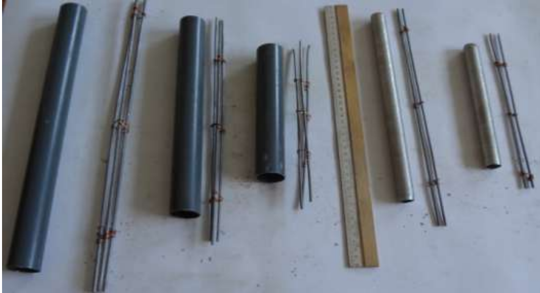
Figure 1. Models of casing bored pile foundations, studied in laboratory studies, with valves.
